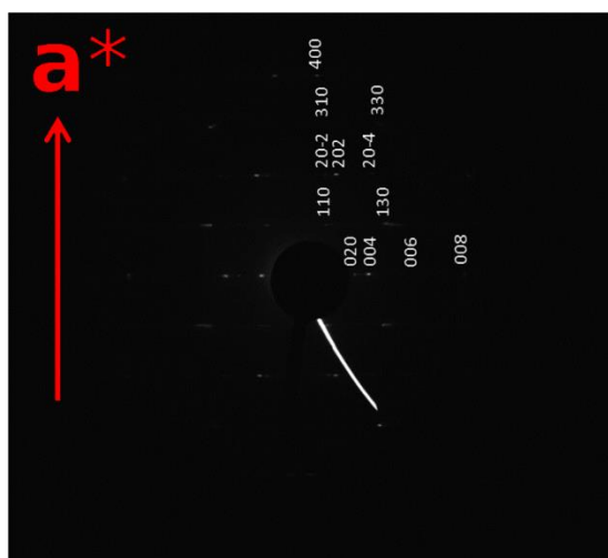
Figure III.37. Electron microscopy investigation of sample 18. TEM/SAED shows a mixed phase constituted by the intimately intergrowth of chrysotile fibres (left) and antigorite blades (right).
