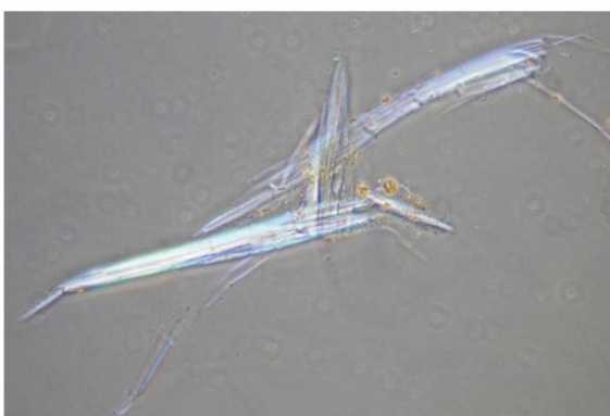
Figure III.34. PLM/DS-PC study of fibrous-lamellae of serpentine. left) RI 1.550 – pale-blue with orange halo ; right) RI 1.5680 – white to pale-blue with soft halo. Fibres exhibit the characteristic staining colours of both antigorite and chrysotile varieties.
